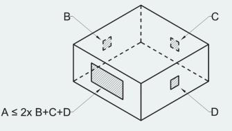
Face treated as dominant where area of openings at that face is at least 2x area of openings in remaining faces
